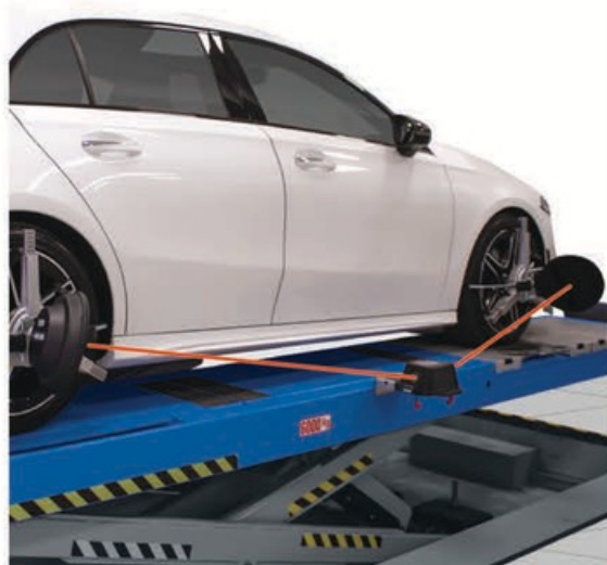
Alinhador 3D móvel multi-câmeras Bluetooth Ravaglioli (made in Italy)
